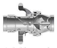
Coupling halves disconnected
